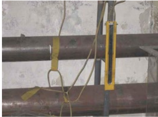
Figure 4. Schematic diagram of the arrangement of the Pitot tube in the air supply duct.
