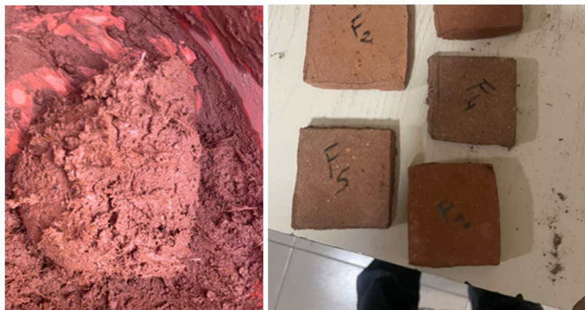
Figure 8. Mixture and samples for the characterization of the asymmetric hot plane.
