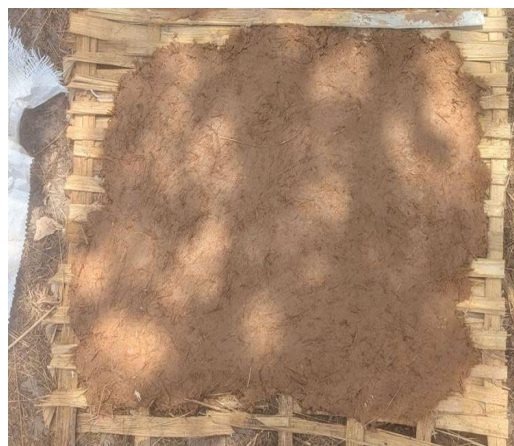
Figure 13. Exploratory application of formulation F4 (7.5% Typha) on the crinting panel.
