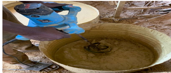
Figure 5. Preparing the clay paste.
