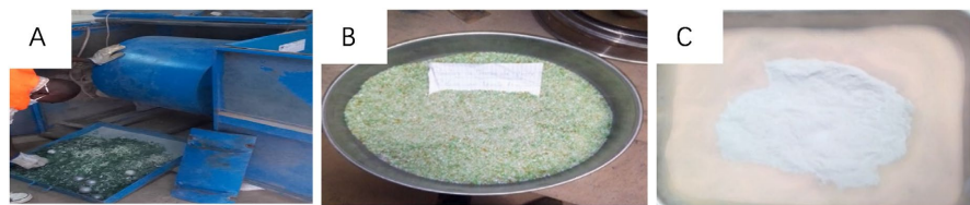
Figure 2. Processing of waste glass: A) crushing, B) screening, C) resulting powder.
