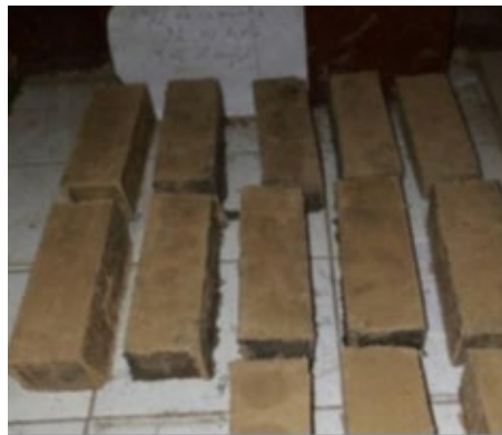
Figure 3. Prismatic test specimen of stabilised soil.
