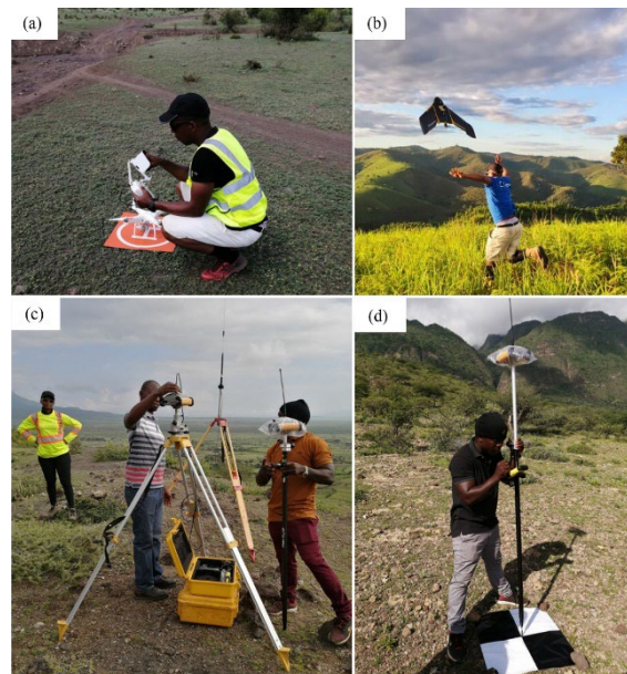
Figure 7. Example UAV data acquisition processes at Engaruka North Terraced Area (ENTA): (a) DJI P4P drone; (b) the same eBee Plus drone used by Tanzania Flying Labs in Engaruka, https://ag.dji.com/newsroom/pilot-story-leka-tingitana ; (c) setting up the RTK GPS land survey equipment; (d) measurement of GCPs.
