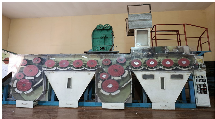
Figure 1. Experimental test bench (schematic configuration with 4 peg-spike drums and 1 saw drum shown).
