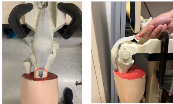
Figure 2. Shows a patella encapsulated in a silicon patella tendon, both front and the side views of the knee joint. The red circle shows the tibial tuberosity.
