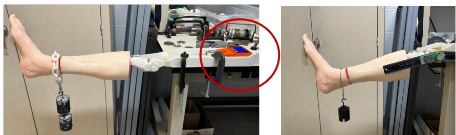
Figure 3. (Left) The side view of the leg at horizontal position (where q = 90^\circ ), the weight is hung at the ankle. Within the circled area, the orange meter is the Newton meter that we used to record the F_t data, (Right) the side view at an angle q = 75^\circ with the vertical.
