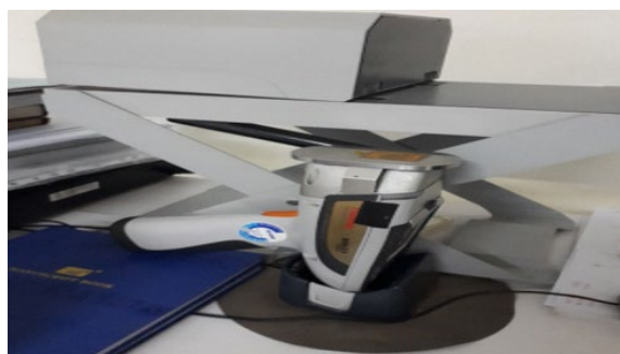
Figure 2. Vertical layout of the Niton XL3T XRF Analyzer.
