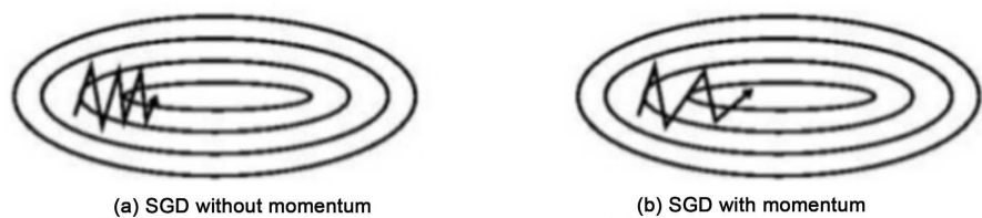
Figure 6. Damping of stochastic-gradient-descent oscillations by the momentum method (SGDM).
