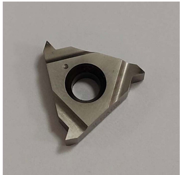
(b) Physical image of the second tool wear test (right tool tip)
